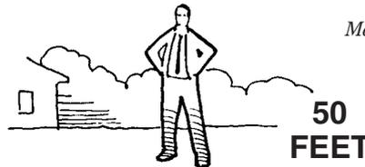
*Reduce the risk of bystanders being struck by flying debris. Make sure no one is within 50 feet (15 meters)—that's about 16 paces—of an operating attachment.*
