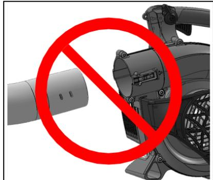
3. Align tabs (C) with grooves (D) and slide straight blower pipe (E) over curved pipe (F) until there is light resistance. Do not force the connection.
