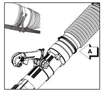
8. Move handle (E) to desired position. Tighten knob (H) hand tight.
