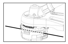
Hold trimmer head while turning 4. knob clockwise to wind line onto spool until about 13 cm (5 in.) of each line remains exposed.
