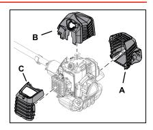
6. Remove grass and leaves from grid (C) between recoil starter and fuel tank.
