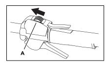
2. Pump purge bulb (B) until fuel is visible and flows freely in the clear fuel tank return line. Pump bulb 4-5 times.
