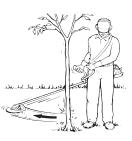
To free a blade that is bound in the cut, stop the engine, and support the trimmer or brushcutter to keep stress off the blade. Push the tree away from the entry point of the cut to open the cut, and pull the blade directly away from the cut in a straight-line motion. Use caution when releasing the tree to avoid being struck by spring-back or falling.
