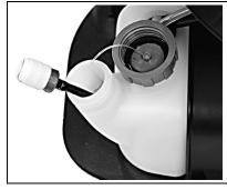
2012 and later gasoline powered engines produced for sale in the United States to be equipped with a special low permeation fuel supply hose between the carburetor and fuel tank. When servicing model year 2012 and later equipment, only fuel supply hoses certified by EPA can be used to replace the original equipment supply hose. Fines up to \$37,500 may be enforced for using an un-certified replacement part.
