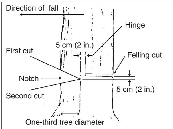
Begin the cut on the side to which the tree is to fall. Cut a notch about 1/3 of the way into the tree. The position of this notch is important since the tree will try to fall "into" the notch.
