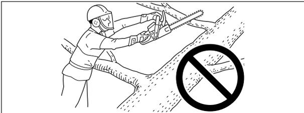
Don't cut with the saw overhead or aligned vertically with your body. If the saw should kick-back, you may not have enough control to prevent possible injury.
