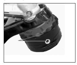
Insert one end of trimmer line into an eyelet, and push line equal distance through trimmer head.
