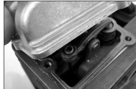
6. Turn engine over several times, and return the to TDC-compression. Recheck with proper feeler gauge to make sure clearance adjustment did not change as a result of tightening the locknut. Readjust as necessary. Use only the type recommended in the Specifications section or an equivalent resistor type spark plug of the correct heat range. Set spark plug electrode gap to 0.6 -0.7 mm.
