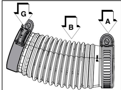
2. Insert anti-static wire through flex tube.
