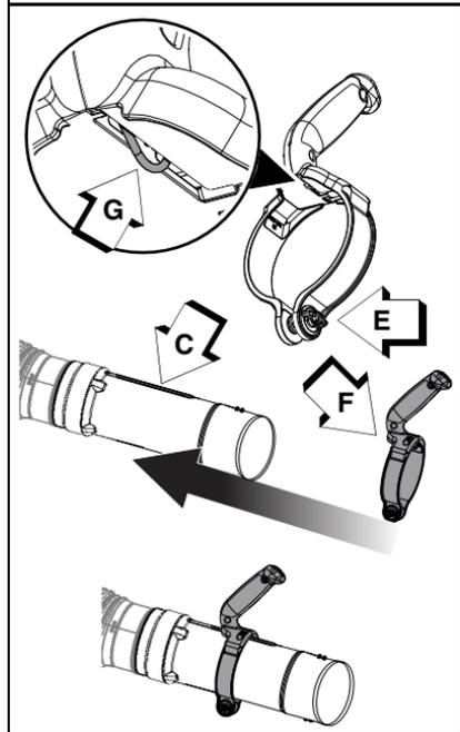
8. Assemble straight pipe (J) onto swivel pipe (C), until you feel light resistance. Hold swivel pipe and turn straight pipe clockwise, engaging positive locking channels, until connection is firm. Do not force connection.
