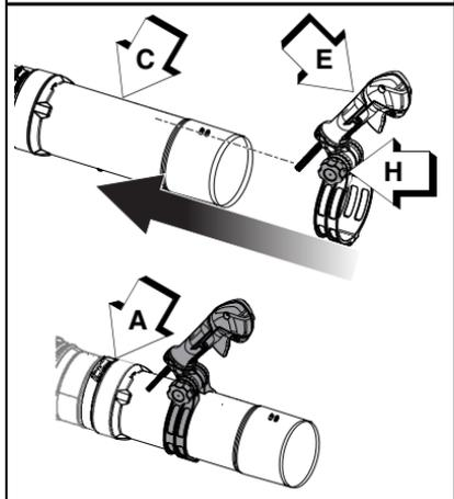
9. Assemble straight pipe (J) onto swivel pipe, until you feel light resistance. Hold swivel pipe and turn straight pipe clockwise, engaging positive locking channels, until connection is firm. Do not force connection.
