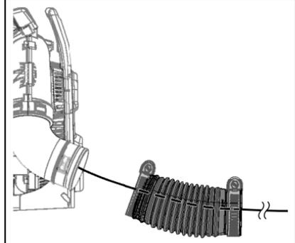
3. Assemble swivel pipe (C) into flexible pipe (B).
