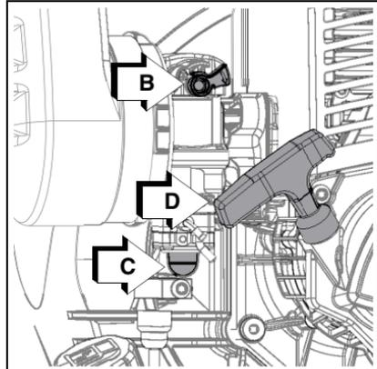
5. If engine fires and remains running, pull throttle trigger (T model) or advance throttle lever (H model) to automatically return choke to run position, then proceed to engine warm up. If engine fires and dies, proceed to step 6.
