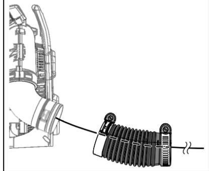
3. Assemble flexible pipe to elbow (D) on blower. Position clamp with cable guide loop (G) on outside of flexible pipe and tighten clamp.
