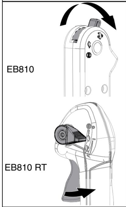
**Note:** If engine does not start with choke in “RUN” position after 5 pulls, move choke to COLD START position, and repeat steps 3- 6.
