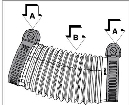
2. Insert anti-static wire through flex tube, into swivel pipe.
