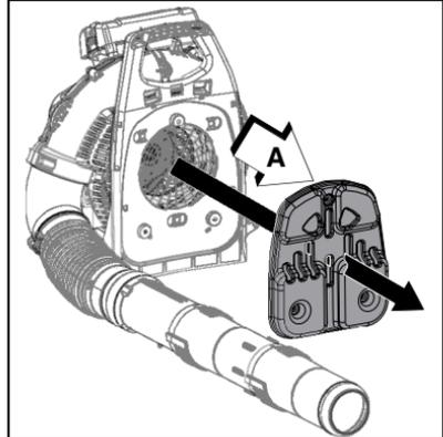
2. Install cold weather insert (B) on frame over air intake.
