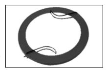
Use blade protectors to protect blade teeth during unit transportation.
