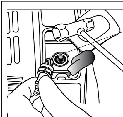
Clean the spark plug and check the gap at the electrode.
