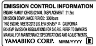
An Emission Control Label is located on the engine. (This is an EXAMPLE ONLY, information on label varies by engine FAMILY).
