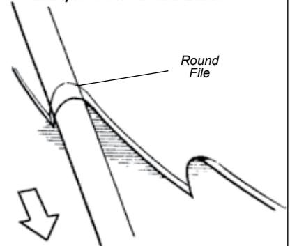
Maintain a radius of 0.04 to 1 to 1.5 mm (0.06 in.) at the base of each tooth. Cutting edges must be offset equally on each side
