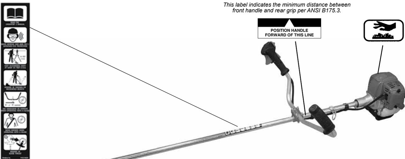
*This label indicates the minimum distance between front handle and rear grip per ANSI B175.3.*
