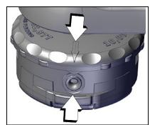
Insert one end of trimmer line into an eyelet, and push line equal distance through trimmer head.
