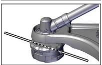
Hold trimmer head while turning knob clockwise to wind line onto spool until about 13 cm (5 in.) of each line remains exposed.
